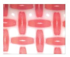
Fig. 10. Top view of the mesh during on-contact screen printing after the fill stroke and prior to snap-off.
